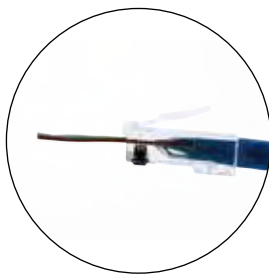
Make sure cable is fully seated. [ STEP 2. ]
