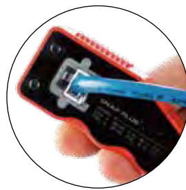
Place assembly into crimping nest. [ STEP 3. ]
